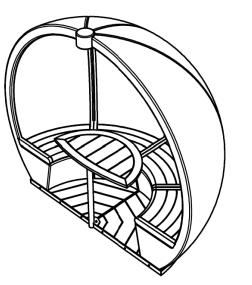
6 person escape pod L2500mm x W2500mm x H2100mm Structure, decking board fit out & seating= 150kg Table & leg= 48kg Solar panel & lights= 11kg Flooring= 56kg
